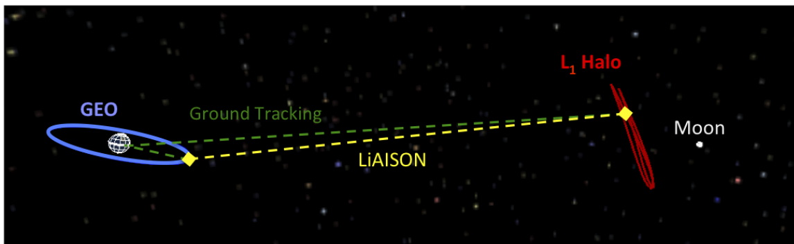
Figure 8.1: Satellite constellation geometry for truth model simulations for LiAISON and ground tracking viewed in the Earth-Moon rotating frame.
